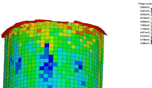
Figure 2: Sample of results for crushing of cylinder
