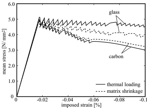
Figure 6: Mean stress-imposed strain relations considering matrix tension softening
