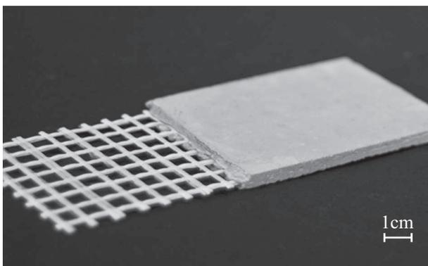
Figure 1: Textile reinforced concrete; photo from Ref. [11]
