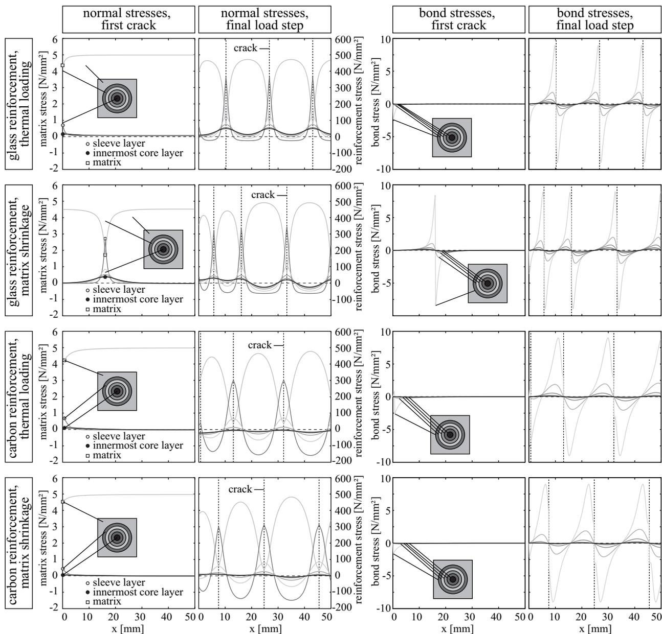
Figure 10: Normal and bond stress distribution on a range of  $0 \leq x \leq 0.05$  m considering matrix tension softening
