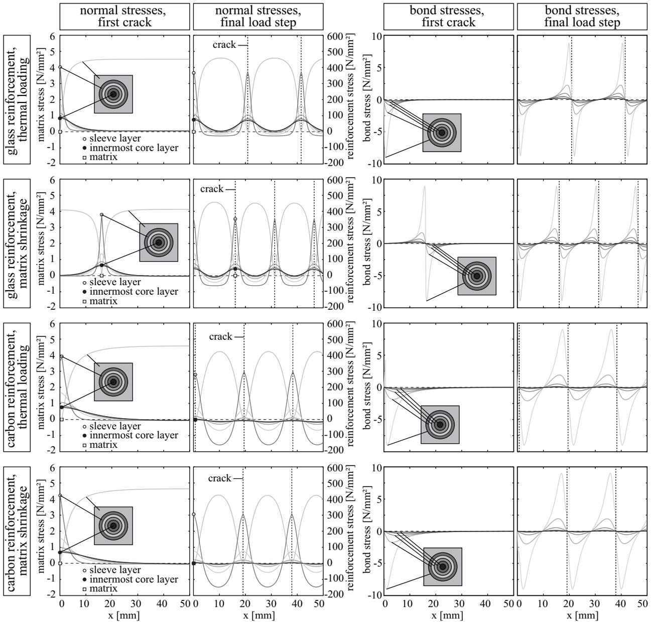
Figure 9: Normal and bond stress distribution on a range of  $0 \leq x \leq 0.05$  m neglecting matrix tension softening
