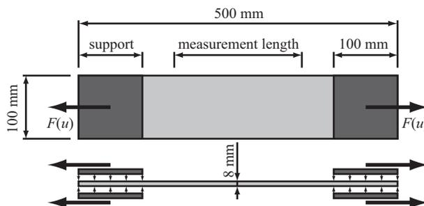
Figure 2: Test setup used by Jesse [14] for the determination of the tensile behaviour of TRC
