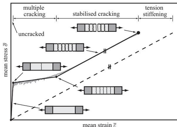
Figure 3: Typical mean stress-strain behaviour of TRC under uniaxial tensile loading; from [11]
