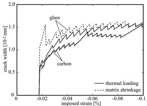
Figure 7: Mean crack width-imposed strain relations neglecting matrix tension softening
