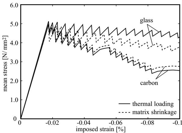
Figure 5: Mean stress-imposed strain relations neglecting matrix tension softening
