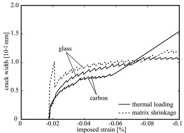
Figure 8: Mean crack width-imposed strain relations considering matrix tension softening
