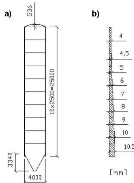
Figure 1: Silo geometry (a) and the sheet thickness (b)
