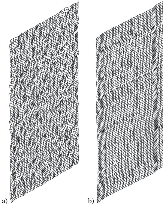
Figure 2: Realizations of the silo initial of the initial geometric imperfection: a) homogeneous field, b) non-homogeneous field
