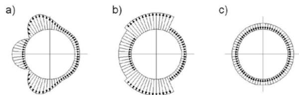
Figure 3: Types of wind loading [1]: a) exact description – trigonometric functions, b) segments loading, c) simplified homogeneous loading
