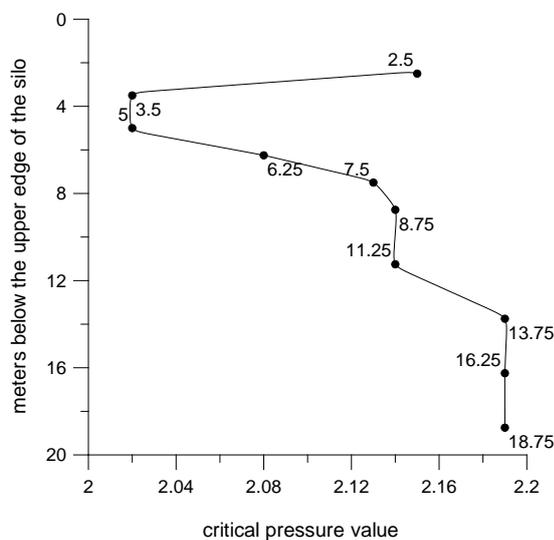
Figure 4: Critical pressure, as dependent on the location of the design code suggested indentation on selected heights
