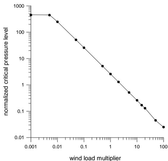
Figure 6: Critical pressure, as dependent on the value of the wind load, normalized on the basis of proper assumptions
