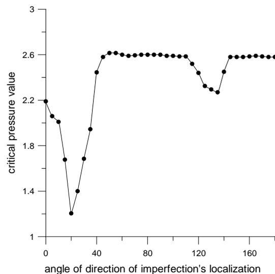
Figure 5: The relationship between the location of a design code corresponding dent and the silo's critical pressure
