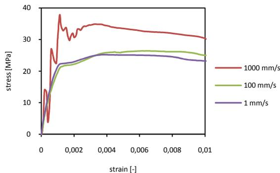
Figure 5: Loading velocity effect
