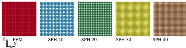
Figure 4: Discretisation of SPH method versus FEM
