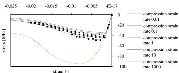
Figure 2: The behaviour of concrete for different strain rates under compression.
