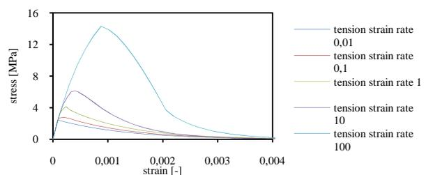
Figure 3: The behaviour of concrete for different strain rates under tension.
