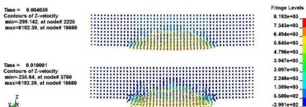
Figure 1: Spalling in concrete slab caused by pressure of 0.1 kg TNT exploded 2 m from the top surface (field of velocity in mm/s).
