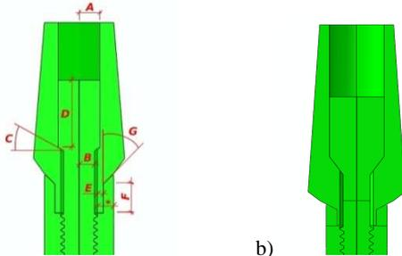
Figure 1: Dental implant geometry: a) the initial model with assumed geometric design parameters, b) the best solution obtained.
