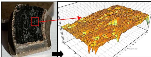
Figure 3: Pad lining sample and surface model
