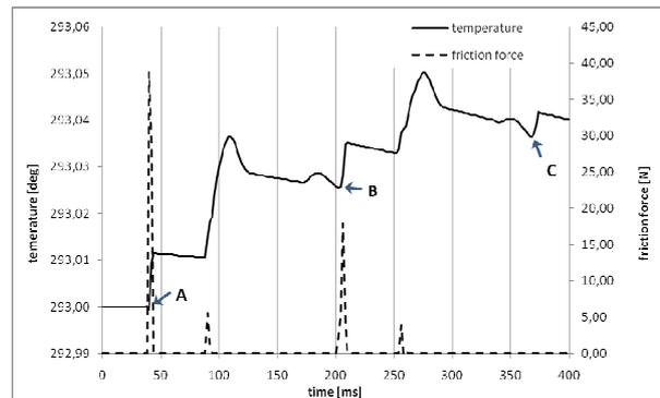
Figure 2: Temperature change in conjunction with friction force
