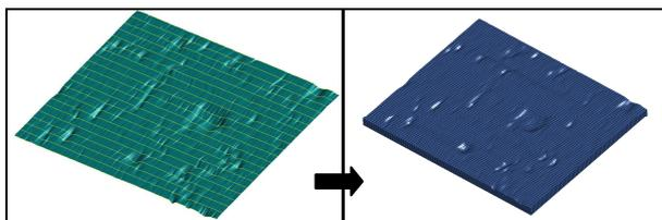
Figure 4: Geometric model and numerical model of microscale friction lining
