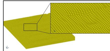
Figure 5: SPH model of brake pad lining
