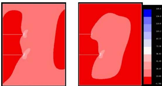
Figure 2:  $\sigma_{22}$  stress distribution in equal and unequal cracks
