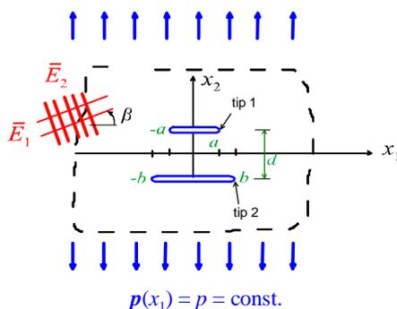
Figure 1: Two parallel unequal cracks
