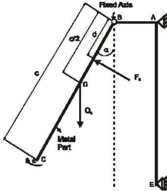
Figure 2: A two dimensional mechanical model of the structure
