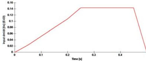
Figure 4: The input mass flow rate curve for the simple airbag model
