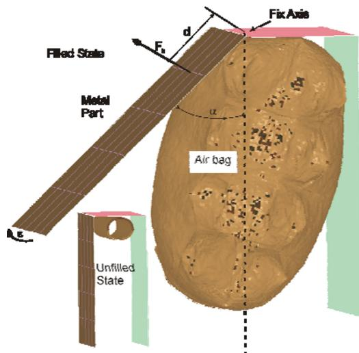
Figure 1: A model of the simple structure for two states: unfilled and filled
