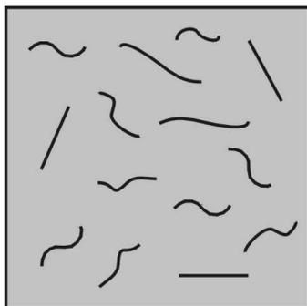
Figure 1: RVE of the carbon nanotube-reinforced composite
