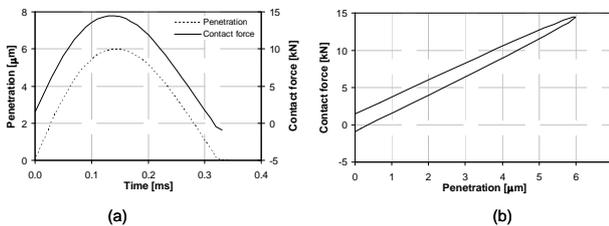
Figure 3: Externally colliding spheres modeled by Kelvin and Voigt contact law: (a) Penetration and contact force versus time; (b) Force-penetration relation
