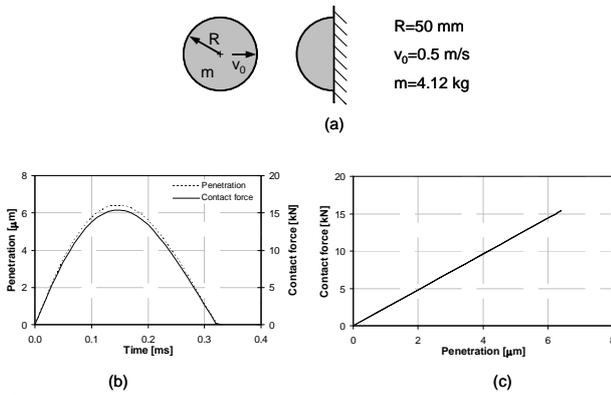
Figure 1: Externally colliding spheres modeled by Hooke contact law (a) Impact scenario of two spheres; (b) Penetration and contact force versus time; (c) Force-penetration relation
