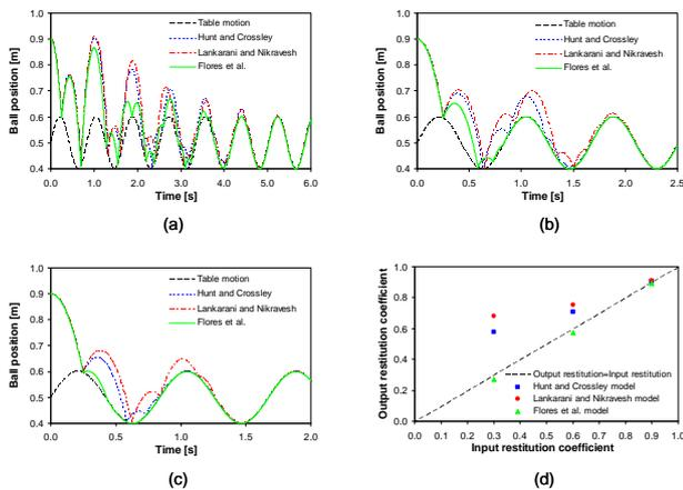
Figure 7: Bouncing ball response for the three dissipative contact force models: (a)  $c_r=0.9$ ; (b)  $c_r=0.6$ ; (c)  $c_r=0.3$ ; (d) Relation between the output and input restitution coefficients
