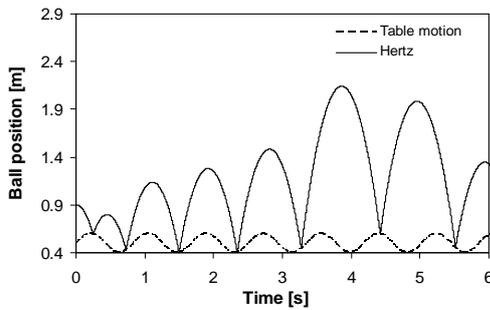
Figure 6: Bouncing ball response for the Hertz contact model
