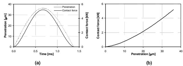
Figure 2: Externally colliding spheres modeled by Hertz contact force law: (a) Penetration and normal contact force versus time; (b) Relation between normal contact force and relative penetration depth
