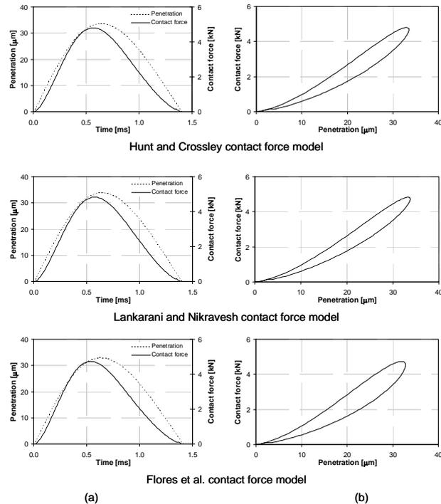
Figure 4: Externally colliding spheres modeled by Hunt and Crossley, Lankarani and Nikravesh, and Flores et al. dissipative contact force models: (a) Penetration and contact force versus time; (b) Force-penetration relation
