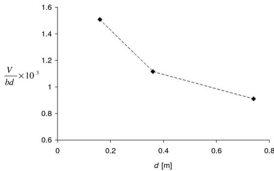
Figure 3: Nominal shear strengths for small, medium and large beams versus beam height
