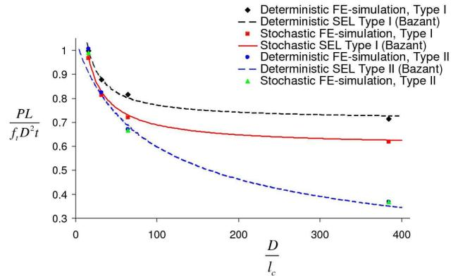
Figure 4: Calculated size effect in notched and unnotched concrete beams compared to model laws by Bazant
