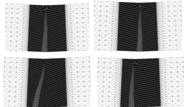
Figure 6: Four arbitrary deformed FE meshes for large-size unnotched beams ( $h=32$  cm,  $u/h=1‰$ ) with random distribution of concrete tensile strength
