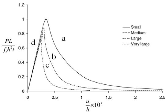
Figure 4: Normalized force-displacement curves with constant values of concrete tensile strength for 4 unnotched concrete beams under three-point bending: a) small, b) medium, c) large, d) very large beam
