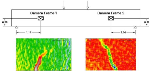
Figure 2: Arrangement of cameras for large beam and measured diagonal localized zones
