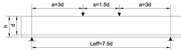
Figure 1: Four-point bending test: geometry and boundary conditions
