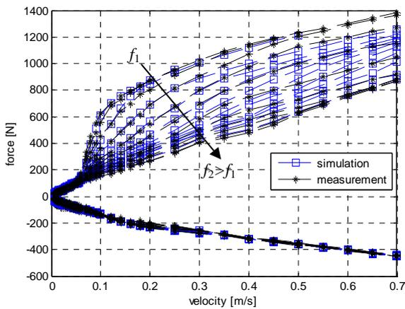
Figure 1: Typical damping characteristic
