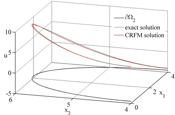
Figure 2: Comparison of the exact solution with the CRFM solution on boundary  $\partial\Omega_2$
