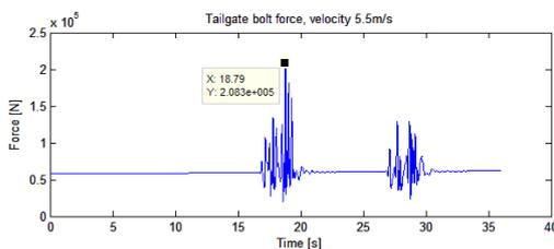
Figure 3: Tailgate bolt force value for real parameters.
