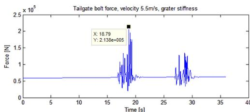
Figure 4: Tailgate bolt force value for grater stiffness coefficient.
