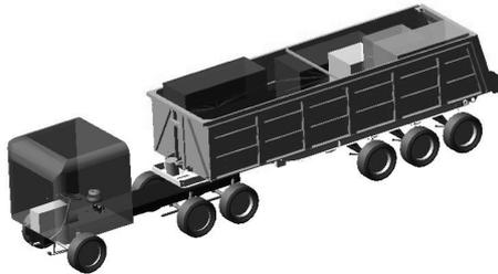
Figure 2: Truck with non-uniform load distributed semitrailer.
