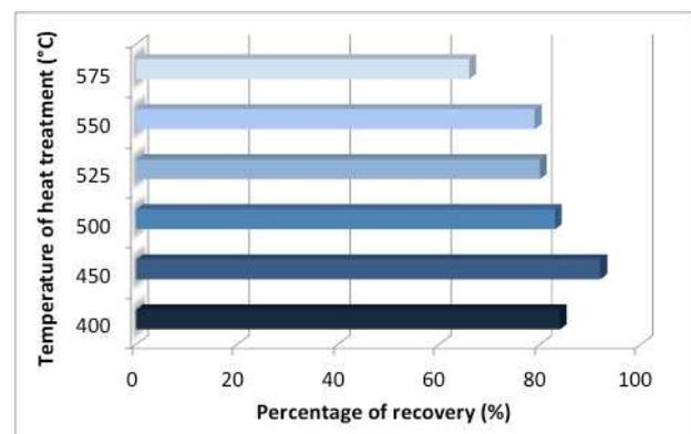
Figure 1: Percentage of recovered shape after heat treatments performed for 25 minutes at different temperatures [6].
