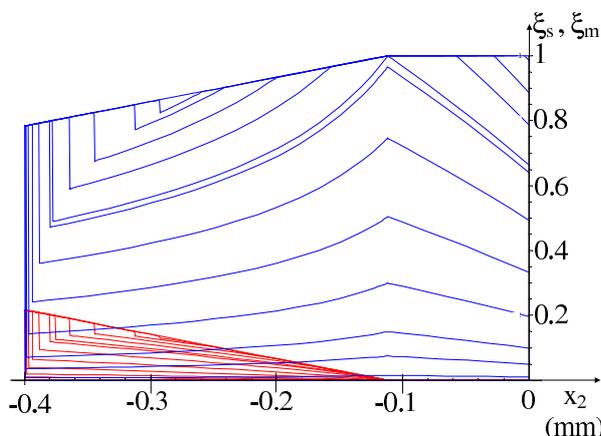
Figure 2: Theoretical twinned martensite (blue line) and detwinned martensite (red line) distribution in the upper half of the beam cross-section at shape recovery [7].
