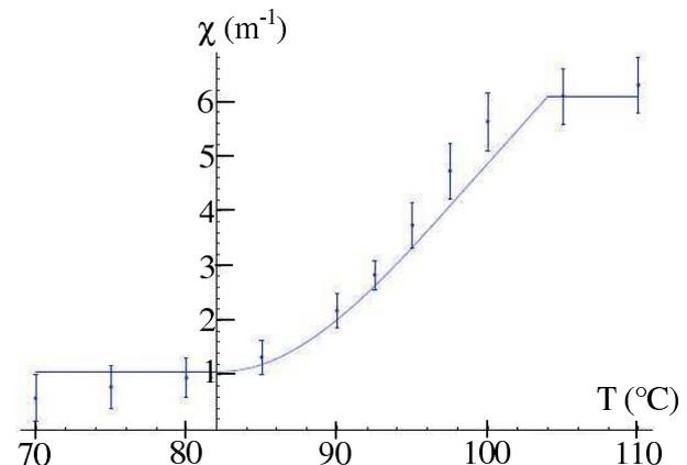
Figure 3: Theoretical curvature-temperature response at shape recovery (solid line), compared with experimental data [7].
