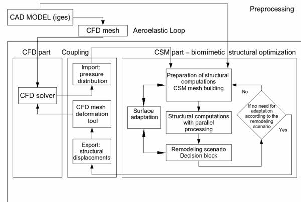
Figure 4: The algorithm for aeroelastic analysis coupled with the biomimetic structural optimization
