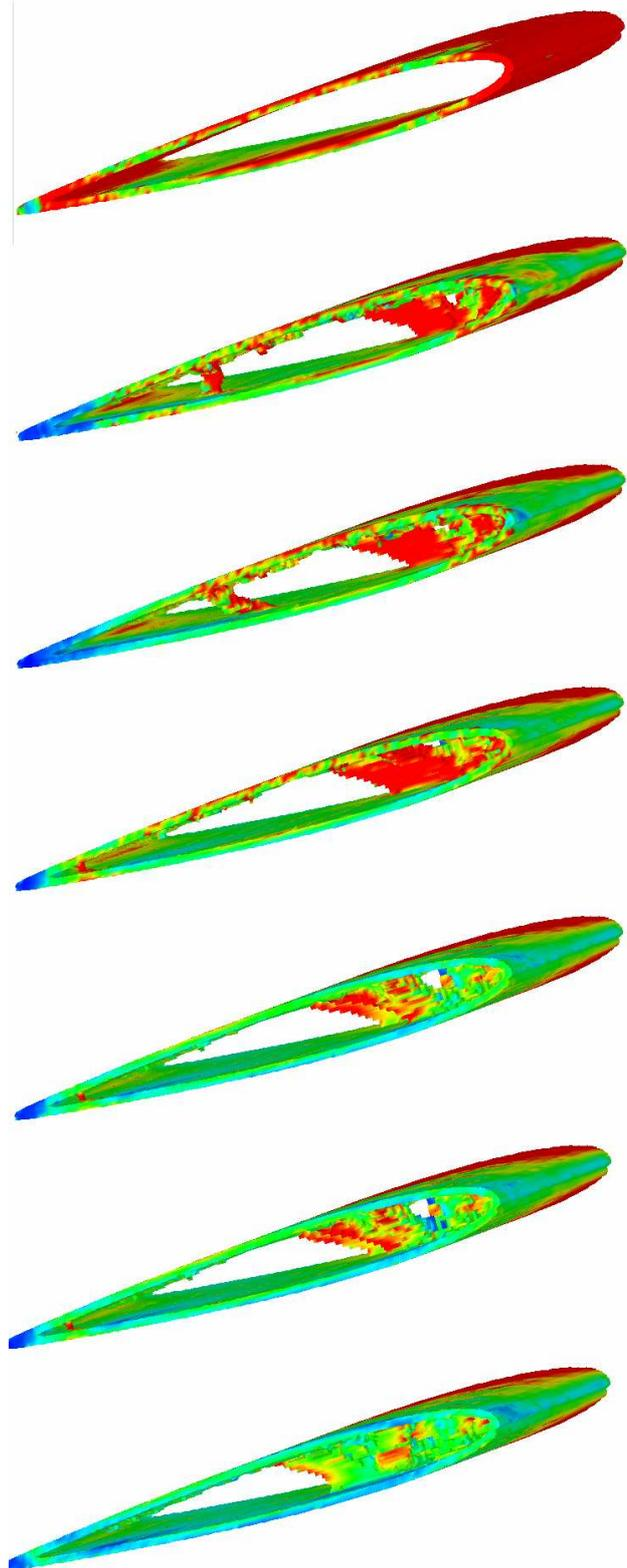
Figure 6: The results of coupled aeroelastic and optimization procedures– from top to down: selected simulation steps.
