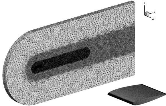
Figure 5: The numerical example - the structural grid for inviscid flow of symmetric NACA0012 airfoil (Mach number = 0.30, angle of attack = 4 degrees, farfield of 20 times long as a chord length).
