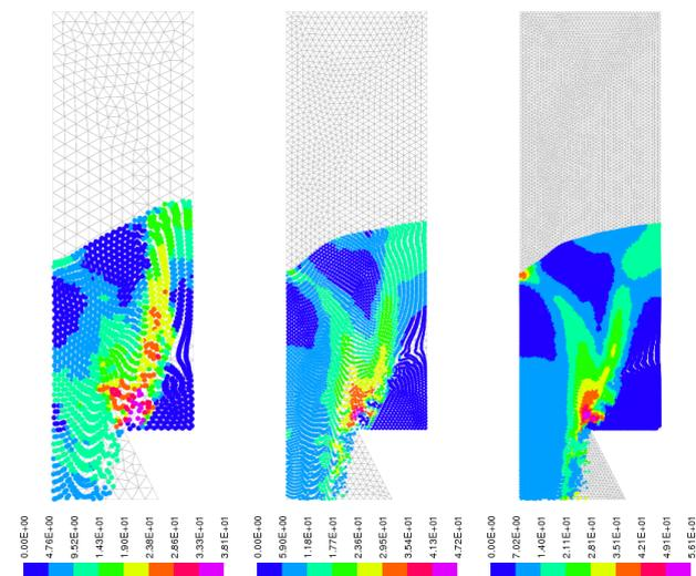
Figure 1: Effective rate of plastic strain (non-local variable), shown for one phase of discharging process (time = 0.25 s). The results are obtained for 3 meshes with different element sizes: 0.01, 0.005 and 0.0025 m
