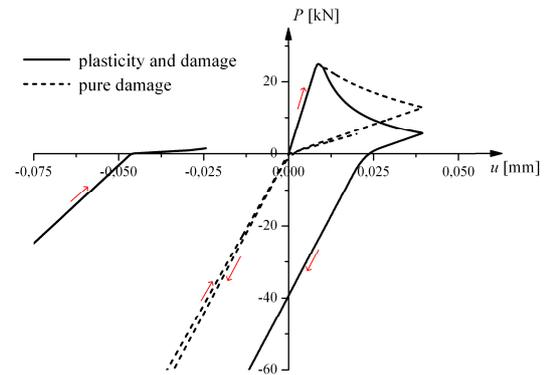
Figure 3: Response of coupled elasto-plastic-damage model during tension-compression-tension test with and without plastic strains
