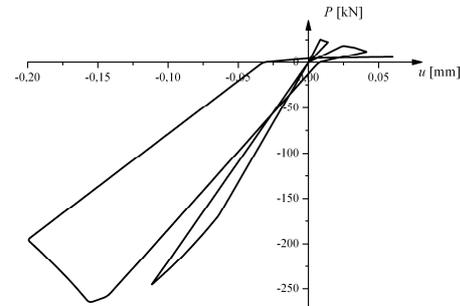
Figure 2: Response of coupled elasto-plastic-damage model for concrete under: a) cyclic uniaxial tension, b) cyclic uniaxial compression and c) tension-compression-tension
