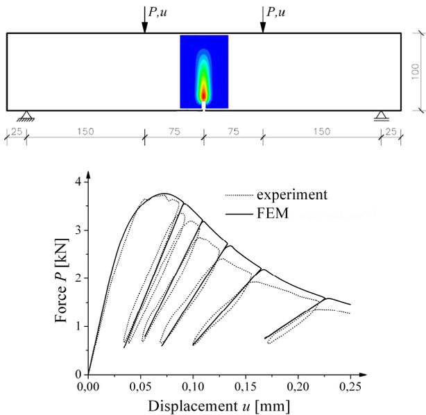
Figure 1: Assumed boundary conditions, calculated localized zone above notch and calculated load-displacement curve compared with experiment [3] for concrete beam
