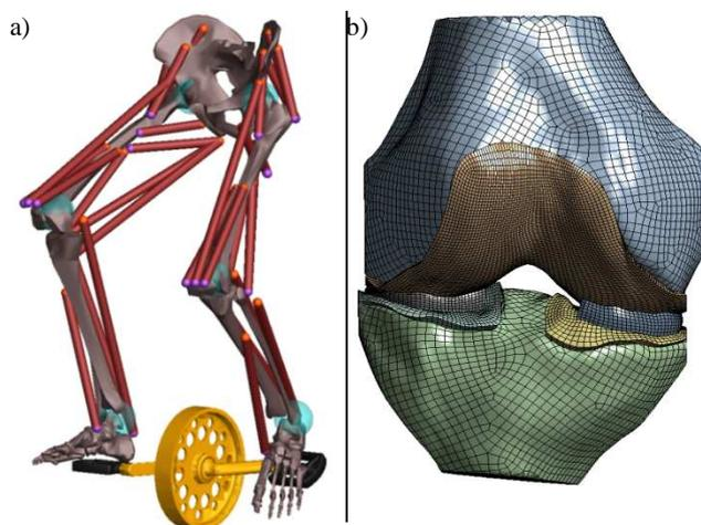
Figure 1: Multibody model (a), knee finite element mesh (b).
