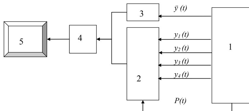
Figure 1: The scheme of arrangement of measuring equipment: 1- models; 2 – tensoamplifier device; 3- scale amplifiers; 4- magnetographs; 5 - personal computer.
