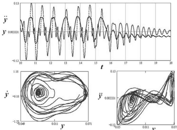
Figure 2: Time processes and phase trajectories of a free oscillation of a rod
