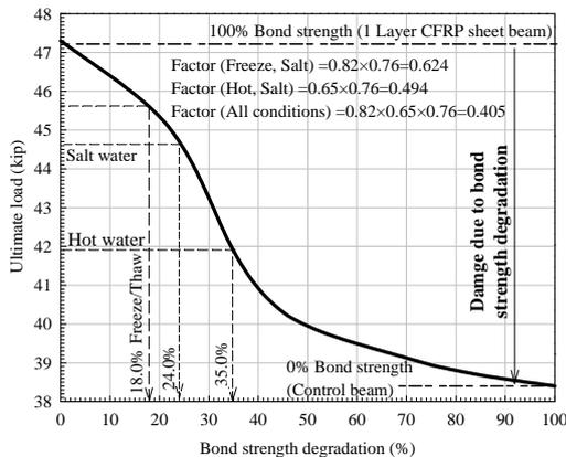
Figure 3: Bond strength degradation vs. ultimate load capacity of control beam.
