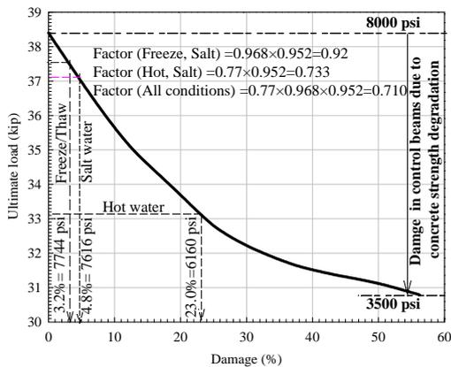
Figure 2: Damage percentages vs. ultimate load capacity of control beam.
