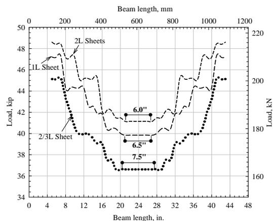
Figure 1: CFRP delamination profile vs. number of CFRP layers
