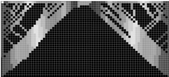
Figure 2: The example of the optimized topology of the truss: free support on left and right sides, homogenous load from top
