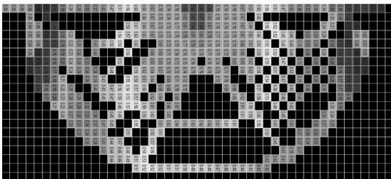
Figure 3: The example of the optimized topology of the truss: free support on left top and right top corner, concentrated force in the middle of the upper edge
