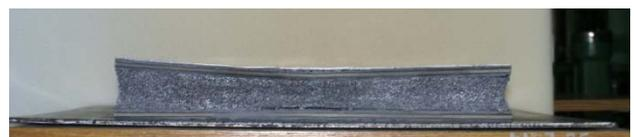
Figure 4: The protective shield – protected plate subsystem removed from the SPS system after the 2 kg TNT explosion
