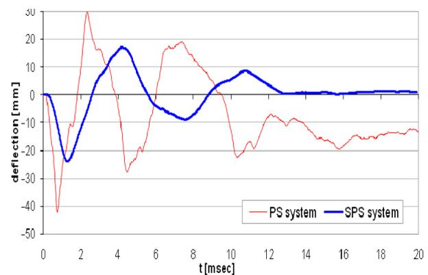
Figure 3: The vertical deflection vs time at the midpoint of the protected plate in reference to the PS and SPS systems under the 2 kg TNT blast shock wave
