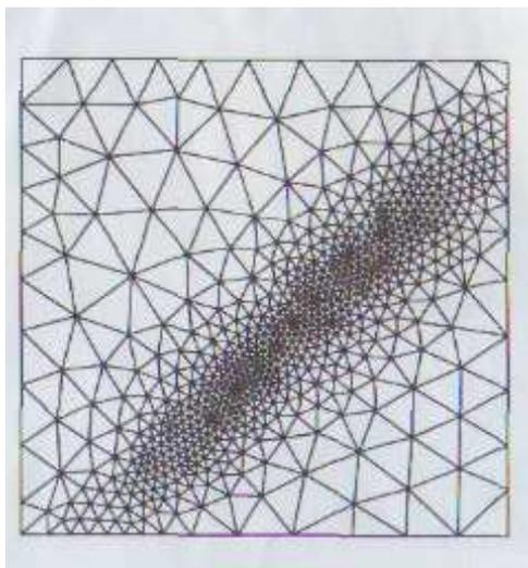
Figure 2: The adapted mesh from the Ref. of O.C Zieniewicz and J.Z. Zhu (1406 elements) [4]
