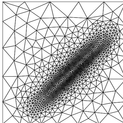
Figure 3: The adapted mesh obtained by the author (1515 elements)
