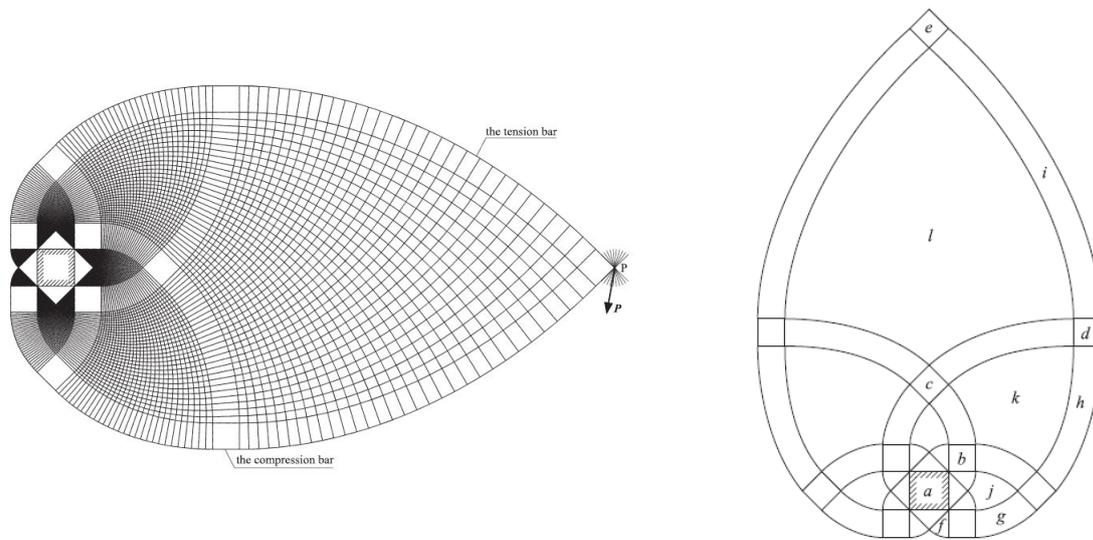
Figure 2: Left: exact analytical optimal Michell truss by Lewinski and Rozvany (2008) and Right: the correctly guessed region topology by Rozvany (1991)
