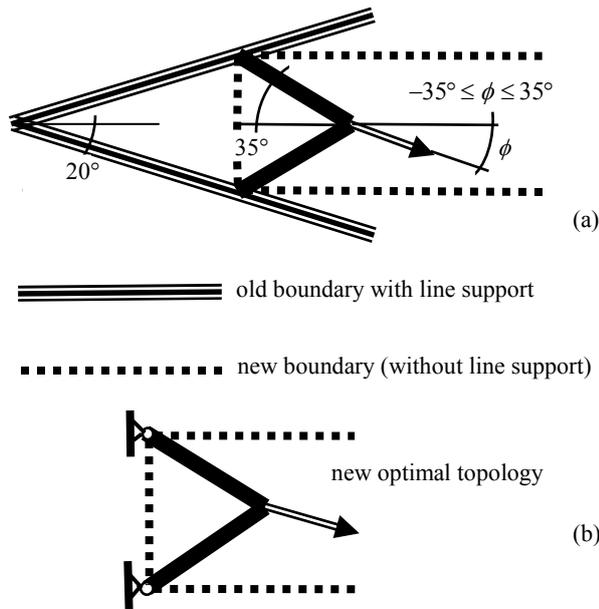
Figure 4: Example for the domain reduction principle
