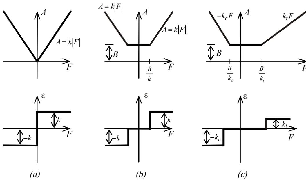
Figure 1: Specific cost functions and the corresponding adjoint strains for trusses with one load condition and a stress constraint: (a) Michell trusses, (a) and (b) equal permissible stress in tension and compression, (b) and (c) prescribed non-zero minimum cross sectional area, (c) different permissible stress in tension and compression
