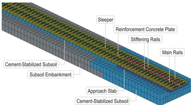
Figure 2. The FE model of the RHEDA track in approach zone
