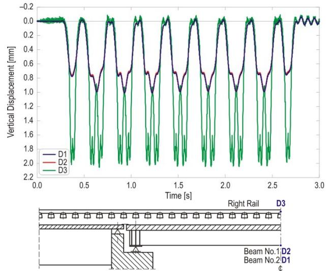
Figure 3. Time histories of selected vertical displacements at the midspan and measurement points in the FE model
