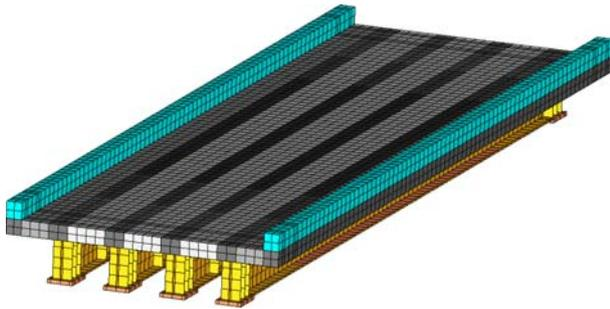
Figure 1. The FE model of the KNI 140070 viaduct superstructure
