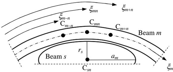
Figure 3: Section A-A across the beam  $s$  at the contact point
