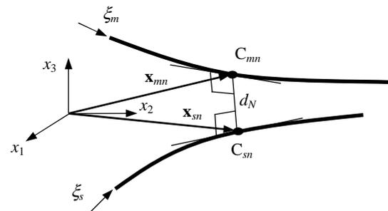
Figure 1: The closest points on contacting beams
