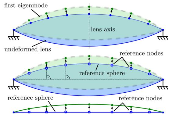
Figure 5: Nodal displacements for the first eigenmode of a lens
