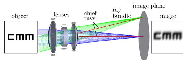
Figure 2: Lens triplet and blurred image due to vibrating lenses
