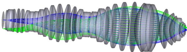
Figure 1: Lithographic projection lens
