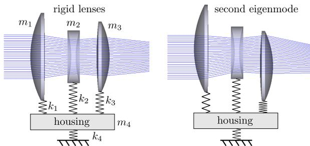
Figure 4: A lens triplet with its mechanical connection to the environment and its second eigenmode
