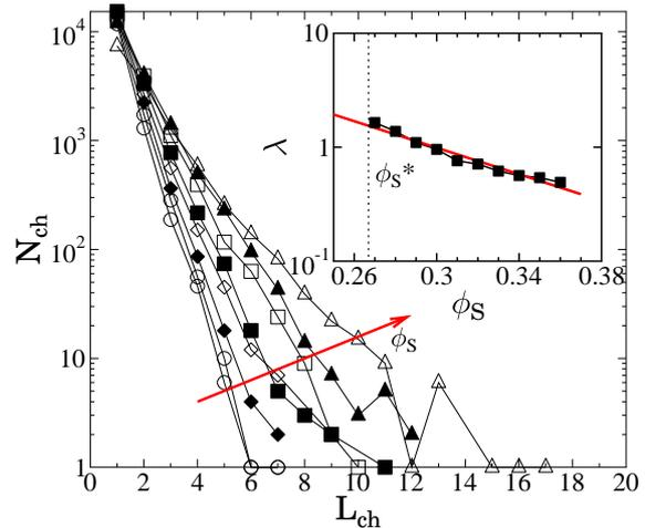
Figure 7: Probability distribution of the chain length on a semi-logarithmic plot. The straight line shows that the functional form is exponential, where the slope depends on the volume fraction  $\phi_S$ . Inset: The coefficient  $\lambda$  is an exponentially decreasing function of  $\phi_S$  for the regime  $\phi_S > \phi_S^*$ .
