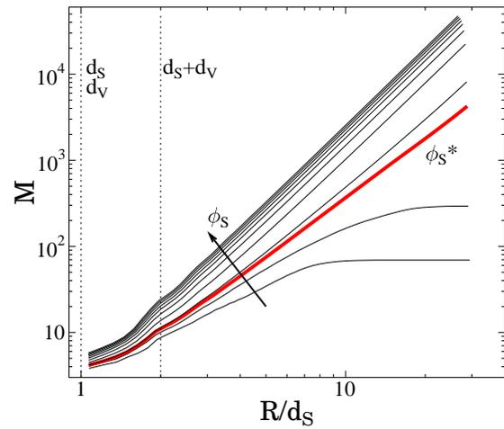
Figure 6: The number  $M$  of particles falling inside spheres of radius  $R$  which are centered on the particles.  $M(R)$  has a power law behavior above the particle size scale. At high concentration the slope of the function is 3 showing the space-filling nature of the cluster, however, close to the critical point  $\phi_S^*$  the cluster proved to have a fractal structure. Here  $d_S$  and  $d_V$  denotes the diameter of the structural and void particles.
