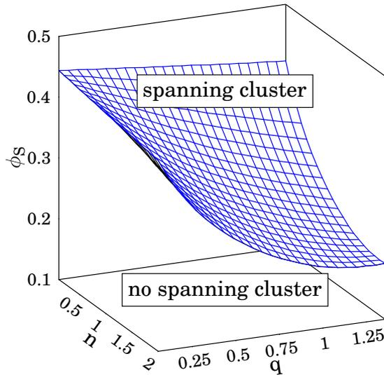
Figure 3: Phase diagram of the system. It can be observed that the percolation threshold can be controlled by varying  $n$  and  $q$ . In the parameter range above the surface a spanning cluster exists, while below it in the sub-critical phase the system is composed of a large number disconnected small sized clusters.
