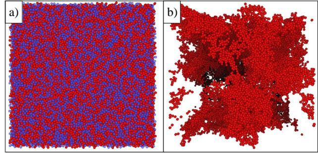
Figure 1: (a) The mixture of structural (red) and void (blue) particles at the end of the construction process. (b) The percolating cluster of structural particles obtained using periodic boundary conditions in all the three directions. Note that the cluster is fully connected even if it has large holes inside.
