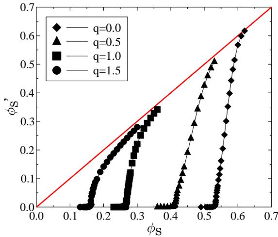
Figure 5: The volume fraction  $\phi'_S$  of the truncated system as a function of initial volume fraction  $\phi_S$ . It can be seen that if  $\phi_S$  is close to the percolation threshold but above it the value of  $\phi'_S$  can be very low as in real aerogels [1, 2, 3]. The continuous red line has slope 1.
