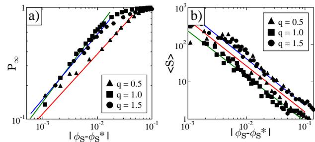
Figure 4: (a) The strength of percolation  $P_\infty$  as a function of  $\phi_S - \phi_S^*$  on a double logarithmic plot at different  $q$  values. (b) The average cluster size  $\langle S \rangle$  as a function of the distance from the critical point. Good quality power laws are obtained for both quantities, where the exponents are independent of the value of  $q$ .
