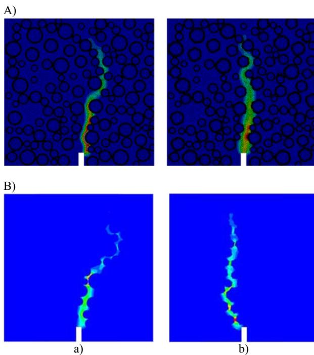
Figure 4: Calculated distribution of non-local strain measure in sand concrete above notch: A)  $\rho=45\%$ , B)  $\rho=60\%$ , a) circular aggregate shape, b) angular aggregate shape and  $l_c=1.5$  mm) [8]
