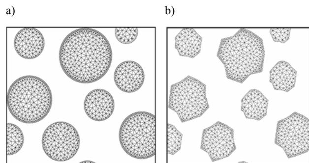
Figure 2: Shape of aggregate used in calculations: a) circular shape, b) angular shape ( $\rho=30\%$ ) [8]
