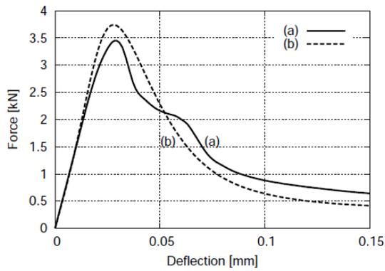
Figure 3: Calculated load-deflection diagram in sand concrete beam: a) circular aggregate shape, b) angular aggregate shape ( $\rho=45\%$  and  $l_c=1.5$  mm) [8]
