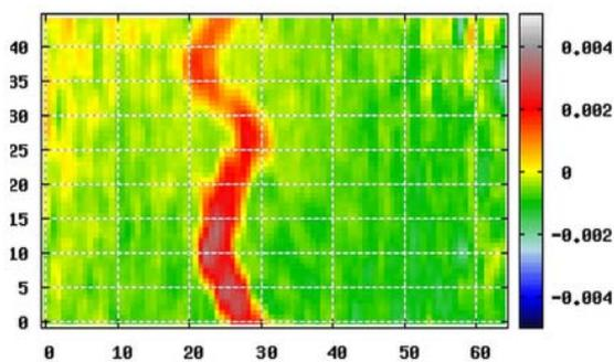
Figure 5: Formation of localized zone above notch in sand concrete beam from DIC [9]
