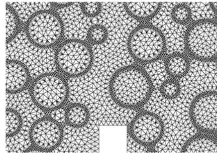
Figure 1: Three-phase concrete in neighbourhood of notch: aggregate of round shape, cement matrix and bond zones [8]
