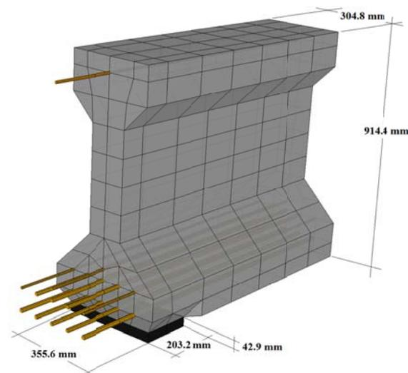
Figure 1: An end part of the FE model of the AASHTO type II girder
