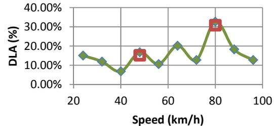
Figure 2: *DLA* vs. speed based on maximum strain on the bottom of girder #4, for the Terex crane in the center of the westbound lane
