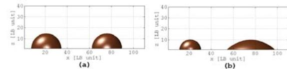
Figure 3: the simulation of the electric field effect on the unstable droplet evaporation process: a) at time=0 and without electric field, b) For a time≠ 0 and with electric field only at the right side.
