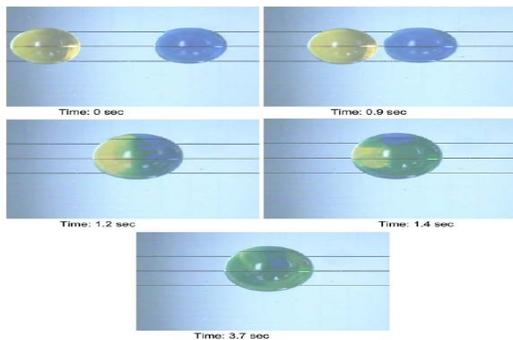
Figure 2: Top views of experimental results for droplets merging  $\theta: 113^\circ \rightarrow 71^\circ$ .
