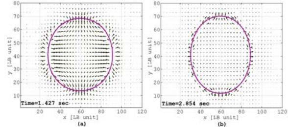
Figure 3: Velocity fields in two times: a) exactly after merging, b) after reaching to equilibrium.
