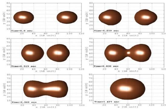
Figure 1: Top views of the simulation of the droplets merging by Electrowetting.
