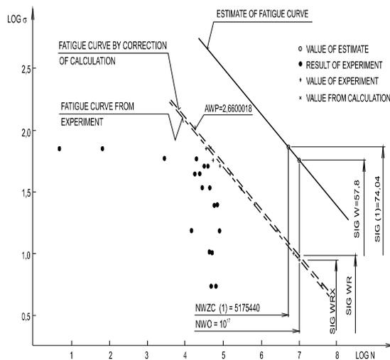
Figure 5: Fatigue curve reduced for tower crane
