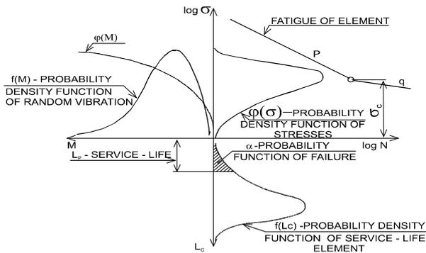
Figure 1: The dependence of a component service life on loading
