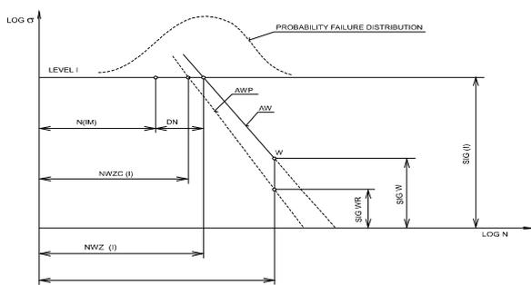
Figure 2: An estimation of a fatigue curve and its reduction
